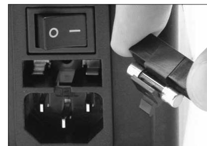
1. Remove the fuse by pulling off the black cap. If necessary use a tool to lever it off.
