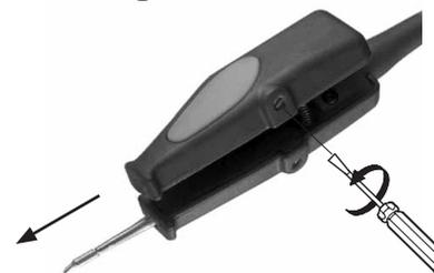
Loosen the screw to remove the cartridge.
